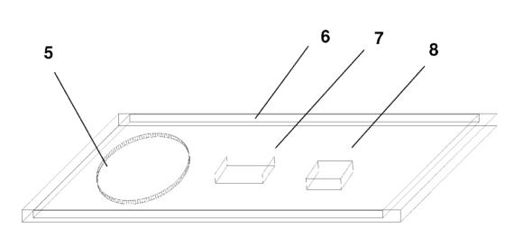
**(57)** Abstract: A sturdy radio tag has an antenna and semiconductor chip tuned to low frequency, encapsulated using a low-temperature, low-pressure, low-viscosity injection molding process.
